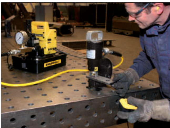
▼ SP-Series, Lightweight Hydraulic Punch – much faster than drilling.
