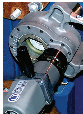
Image above: alkitronic® CLS-SG in operation on a plate heat exchanger.
