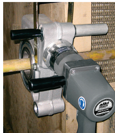
Image above: alkitronic® RCL pneumatic torque multiplier in operation on a plate heat exchanger.
