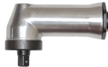
4UA9 03070216 1/2" right-angle head (speed reduction: 25% torque output reduction: up to 50%)
