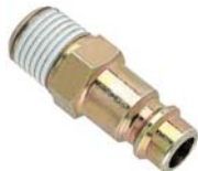
77NMC4 88104096 7N7/7S7 Series nipple, 1/2" male thread, 7,2 mm bore (EURO 7,2 - 7,4)
