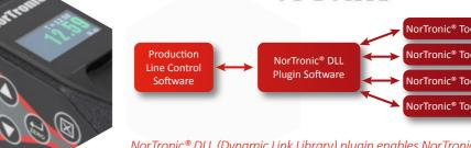
NorTronic® DLL (Dynamic Link Library) plugin enables NorTronic® 868 MHz and 915 MHz version tools to be interfaced to a customer's existing production line control software. DLL is not compatible with Bluetooth® versions. Contact Norbar for more details.
