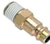
77NMC4 88104096 7N7/7S7 Series nipple, 1/2" male thread, 7.2 mm bore (EURO 7.2 - 7.4)
