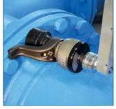
Improved reaction arm. Drop-forged reaction arm with lock on function, made of light chrome vanadium steel alloy for durability, stability and performance. It is equipped with an offset reaction arm and can be retrofitted with a straight reaction arm
