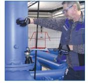
Overload safety. An integrated overload safety mechanism protects the gear unit, by ensuring that the square drive has a pre-determined breaking point. The square shears if overloaded and is easily replaced
