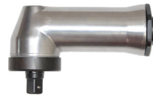
4UA9 03070216 1/2" right-angle head (speed reduction: 25% torque output reduction: up to 50%)
