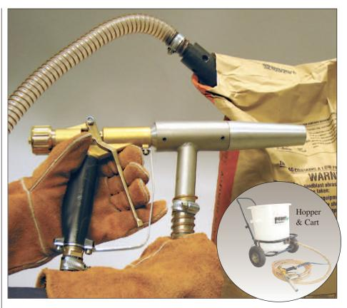
gun. The vacuum draws abrasive through the hose into the gun, where it mixes with compressed air. The air-abrasive mix exits the gun and strikes the surface to be blasted.
