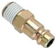
IB6NMC3 88103023 IBN/IBS Series nipple, 3/8" male thread, 6 mm bore (ISO6150B / MIL-C4109)
